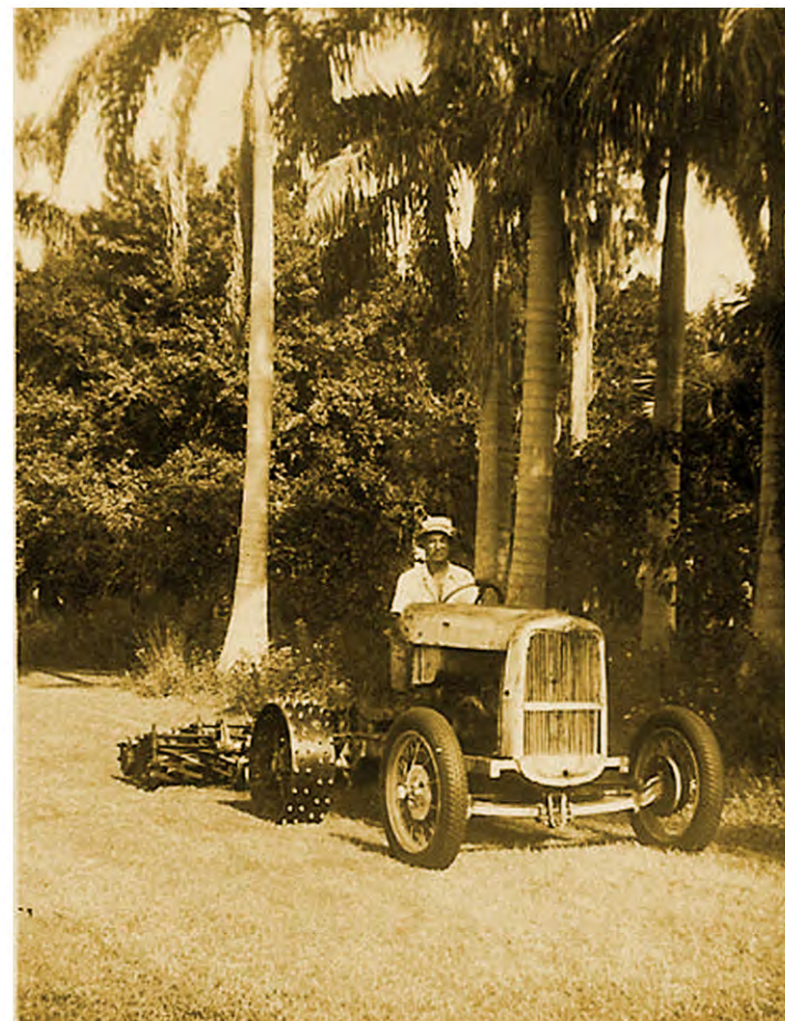
George Richardson, Sr. on a 1930's Worthington Golf Tractor. These tractors were made primarily from Ford Model A/B automobile engines, running gear and other parts.
